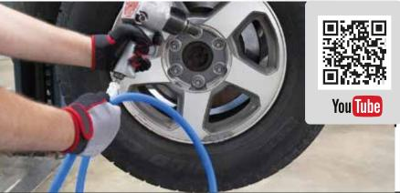
BluBird hoses are 40% lighter, stronger and more flexible than other rubber hoses. BluBird hoses have superior cold weather flexibility down to -50°F and maintains its integrity up to +190°F making it a year round hose in most parts of the world. BluBird hoses have an abrasion resistant external cover combined with high strength woven polyester reinforcement to prevent elongation and added strength giving BluBird hoses a 300psi working pressure and a 4:1 safety burst factor.
